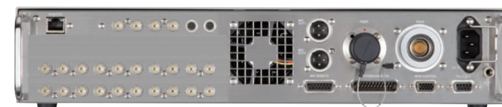
CU-HD1300FT Rear Panel (Fiber/Triax)
