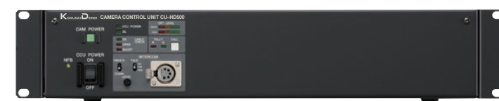
CU-HD500 Front Panel
